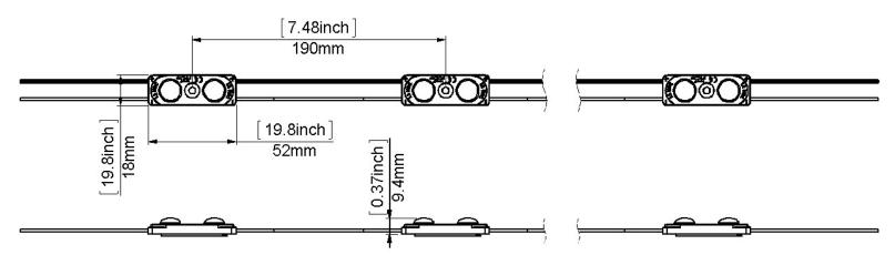
\* Client can customize the modules distance (center to center) based on requirements.
