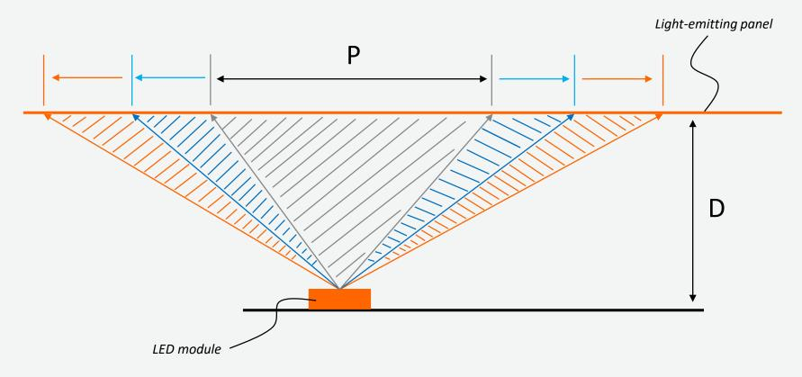
The proportion of "P" and "D" can show the performance of lens design, normally, the bigger proportion, the larger light spot.
