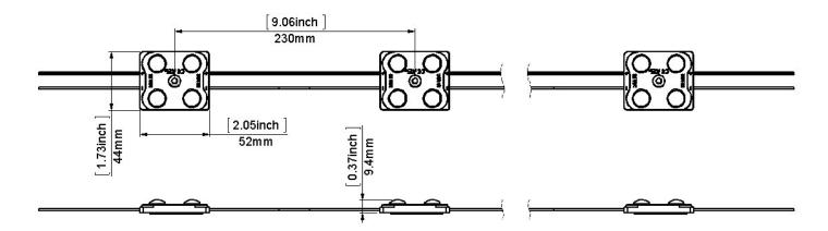
\* Client can customize the modules distance (center to center) based on requirements.
